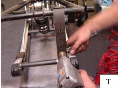
17. Remove the upper shock bolt, then remove the lower shock shaft by removing the bolt on each rail. retain ALL loose parts for re-use.(Pic U,V)
