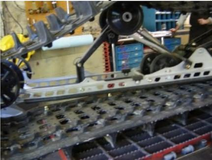
24. align front arm with mounting point on your tunnel, insert bolt and torque to 35 ft. lbs.
