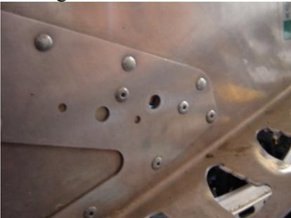
25. Align rear arm with mounting points on the drop brackets, insert bolt and torque to 35 ft. lbs.
